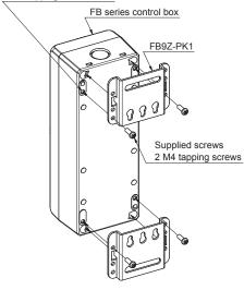
·Using two M6 screws, fasten the FB9Z-PK1 securely on the frame.
